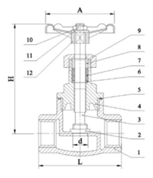
ASTM A351 CF8M 316 Stainless Steel Body, Bonnet and Disc.
